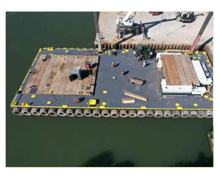
**TM-9** STEEL-HULLED SPUD BARGE
