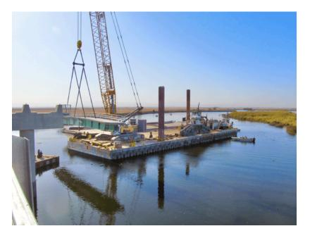
MORTY STEEL-HULLED SPUD BARGE
